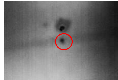
Indication at a fastener under a layer overlapping
