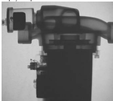
Figure 2.54: Thermal/cold neutron radiography of an oil-filled pump.
