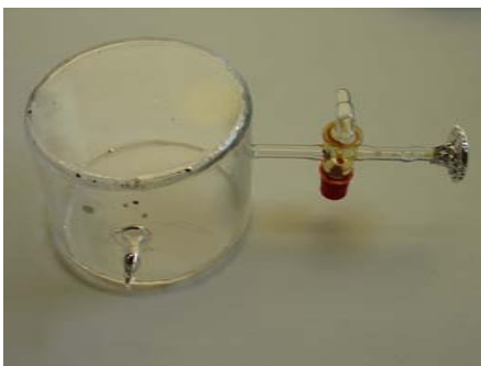
Figure 1.11: NSF cell coated with metallic Cs.
