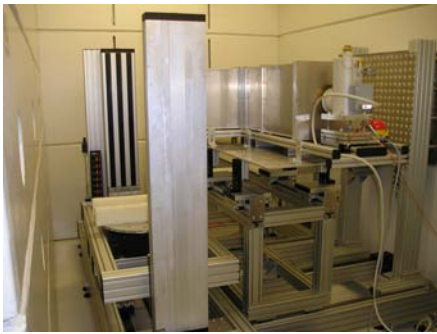
Figure 2.42: Photograph of the NECTAR facility. Left: Manipulator for the samples. Right: Detector system based on a liquid nitrogen cooled CCD camera.
