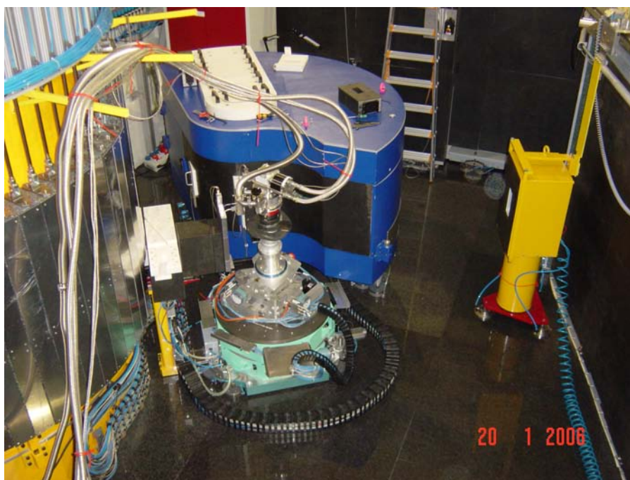
Figure 2.38: View on the triple axes spectrometer PUMA within the experimental hall of FRM-II.
