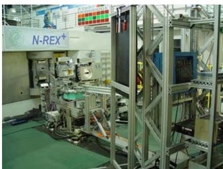
Figure 2.34: The neutron/X-ray reflectometer N-REX + in its present state. The open structure between monochromator, sample and detector allows adoption of extended beam conditioning equipment, e.g. a SERGIS set-up.
