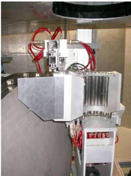
Figure 2.28: The detectors as mounted in the instrument chamber. On the left there is the chopper vacuum chamber.
