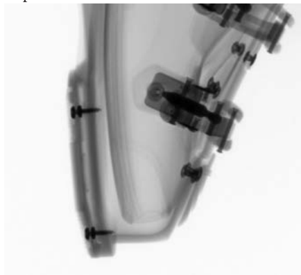
Figure 2.60: X-ray radiography of a ski boot.
