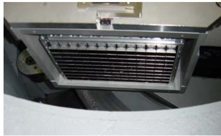
Figure 2.39: PG(002) monochromator within the change unit in the primary shielding.
