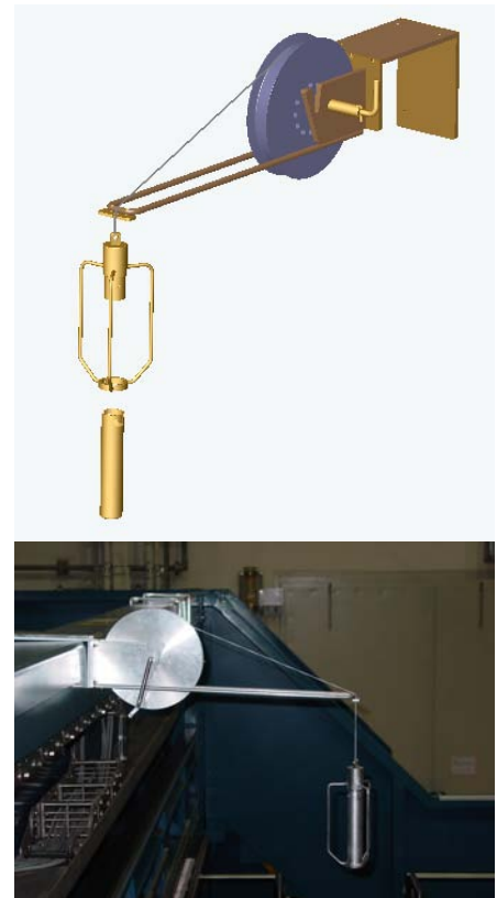
Figure 2.21: Design of the irradiation device for the fishing irradiation position.
