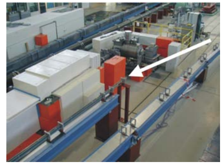
Figure 2.50: End position of the S-shaped neutron guide NL 4a for the SANS-1 instrument.
