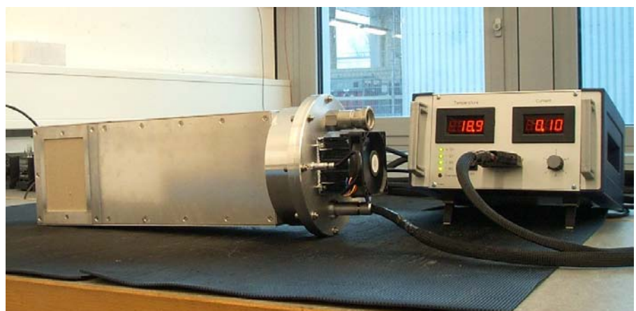
Figure 1.8: 6 LiF/ZnS scintillator based neutron camera with optical CCD-readout.
