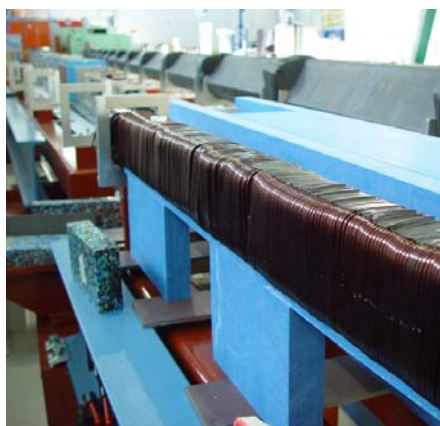
Figure 1.18: The last part of the NG NL2a-o before the selector gap during the installation period. The glass elements are surrounded by the magnetic coil windings. The NG directly behind the NL2a-o is already enoused with 10cm thick PE plates.
