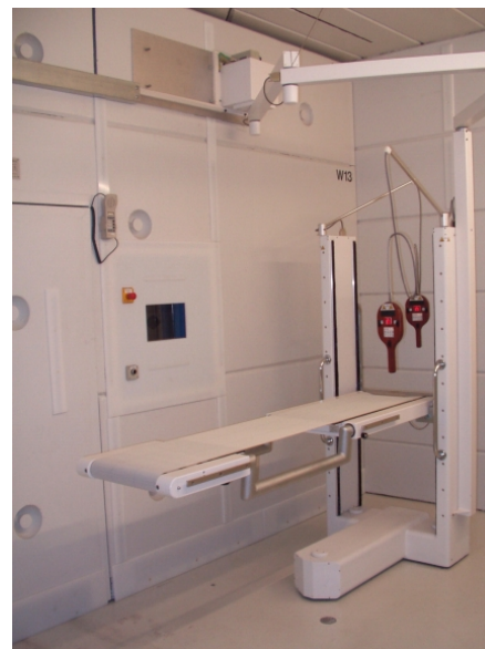
Figure 2.65: The medical irradiation room with the collimator exit and the treatment couch.
