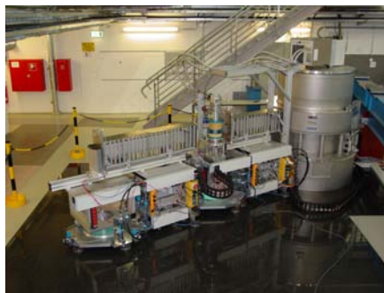
Figure 2.7: Mira equipped with a magnet and a cryostat. In order to reduce scattering by air, the neutrons travel in evacuated tubes before and after the sample.
