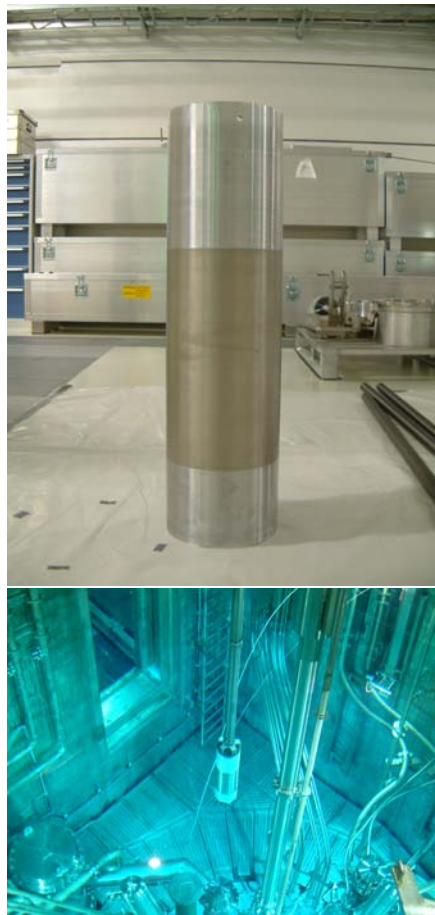
Figure 2.23: top) Ni-liner after the coating, bottom) Test doping rig mounted with the first nickel liner after an irradiation in the reactor pool.
