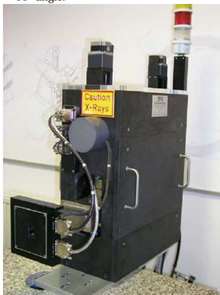
Figure 2.37: The compact-source unit of the add-on X-ray reflectometer (EFG, Berlin). This machine can deliver Cu-K \alpha radiation of variable divergence. The beam is rotated around the sample by means of two vertical translation stages. Therefore neutron and X-ray characterization can be performed simultaneously without mutual interference.
