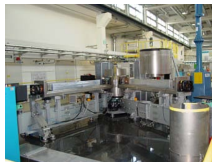
Figure 2.66: The image shows the two secondary spectrometer arms of RESEDA. The open mumetal shielding gives free view on the NSE and NRSE coils.
