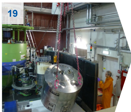
19 Old beam plug nearly ready to leave the Experimental Hall.
