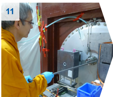
11 Dismantling its drive shaft.
