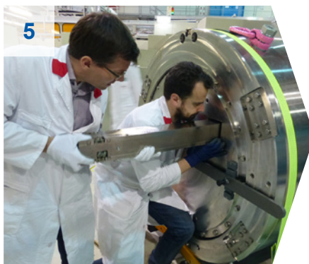
5 The Neutron Optics Group inserting the new neutron guides.
