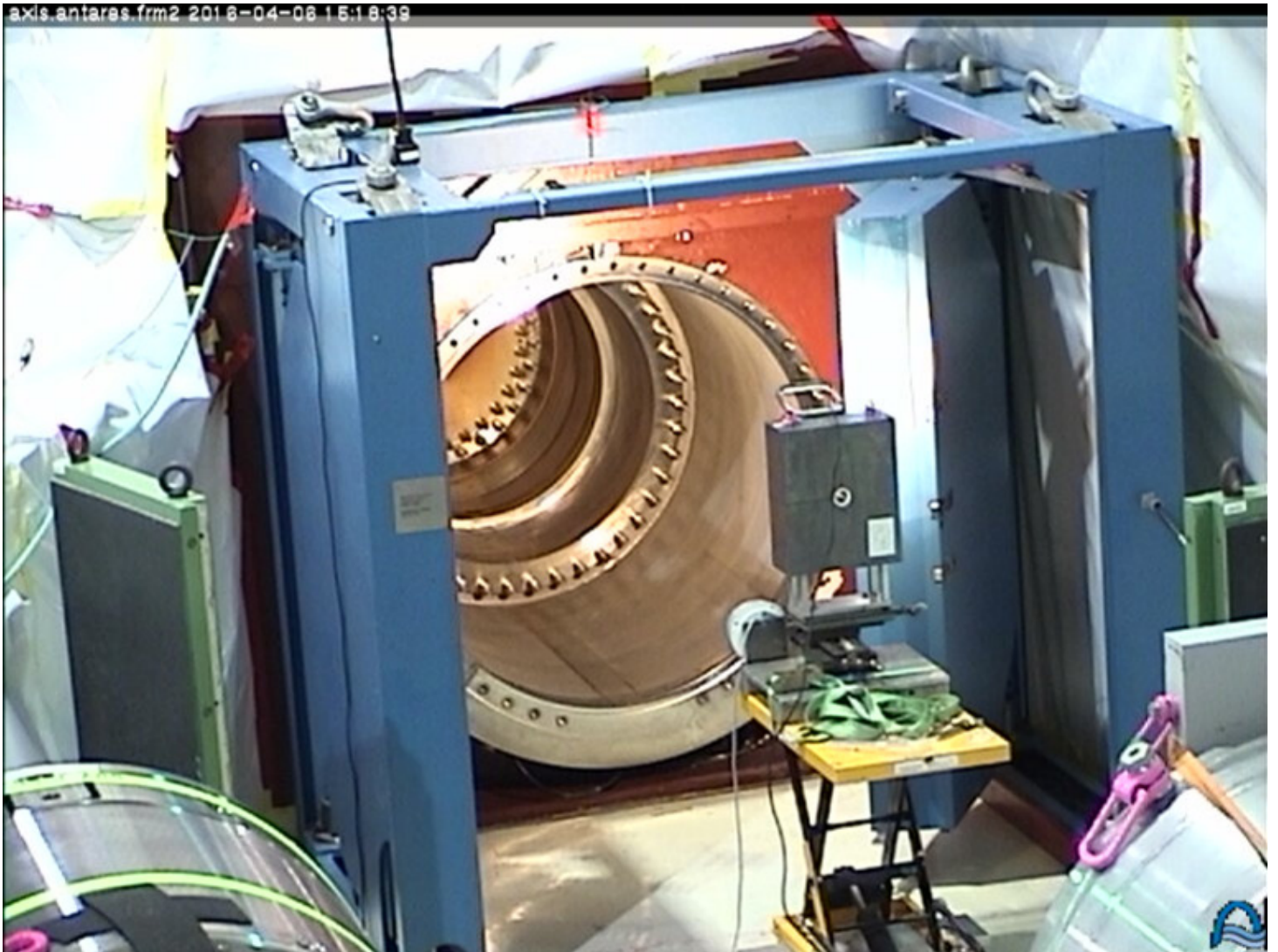
Maybe not the best photo from an artist's view, but a really rare one: The open reactor wall after removing the old beam plug.
