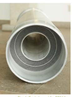
The fuel element of the FRM II is a hollow cylinder of some 1.3 m in length, 24 cm diameter and with a total weight of 53 kg. It contains approximately 8.1 kg of uranium enriched to 93 % of the fissile uranium <sup>235</sup>U. The fuel in use is  $U_3Si_2$  dispersed in Al.
