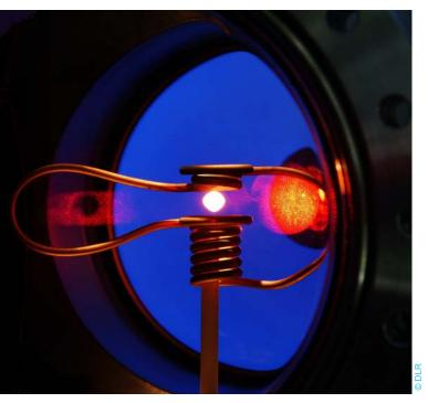
Fig. 1: Levitating metallic droplet, processed by electromagnetic levitation (EML).
