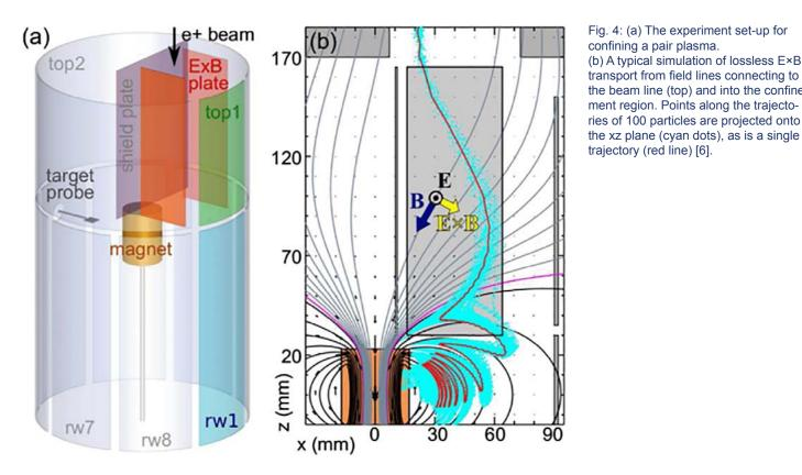
Fig. 4: (a) The experiment set-up for confining a pair plasma. (b) A typical simulation of lossless E×B transport from field lines connecting to the beam line (top) and into the confinement region. Points along the trajecto-
