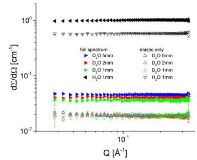
Fig. 2: The measured scattering cross section of  $H_2O$  and  $D_2O$  when full scattering spectrum or only the elastic scattering are considered.
