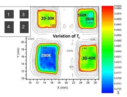
Fig. 2: 2D-S-parameter map of four 200 nm thin YBCO samples obtained by spatially resolved DBS (positron energy: 4 keV). The variation of the S-parameter (colour code, right) allows the determination of the local  $T_c$  inside the individual samples.
