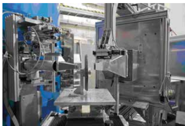
Figure 2: Slit-system for residual stress analysis.
