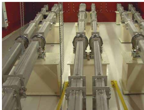
Figure 3: Neutron guides inside the neutron guide tunnel.
