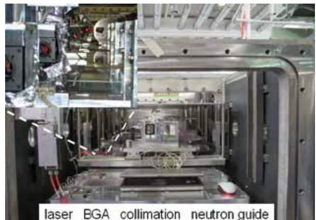
Figure 1: View into the collimation chamber of the SANS-1.
