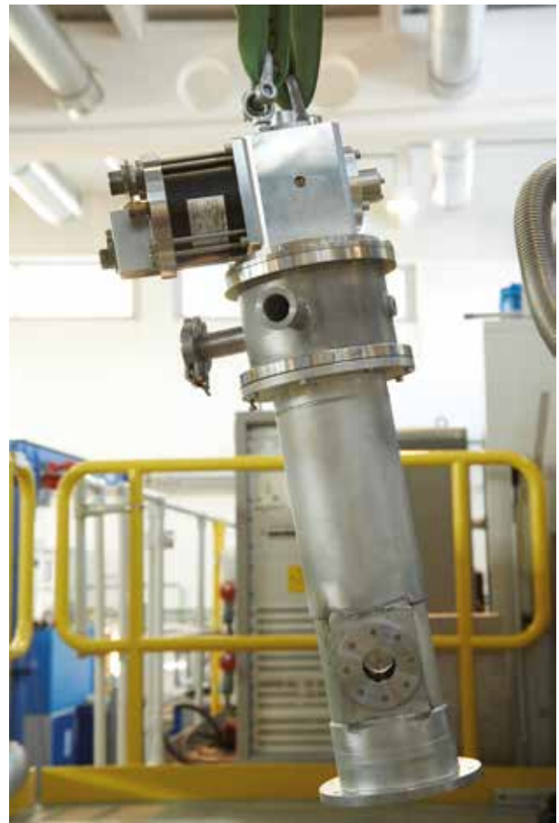
Figure 2: Cryostat with sapphire window (in detail on the left).
