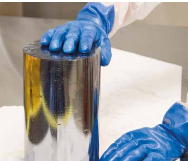
Figure 1: A silicon crystal after the doping at the FRM II neutron source.
