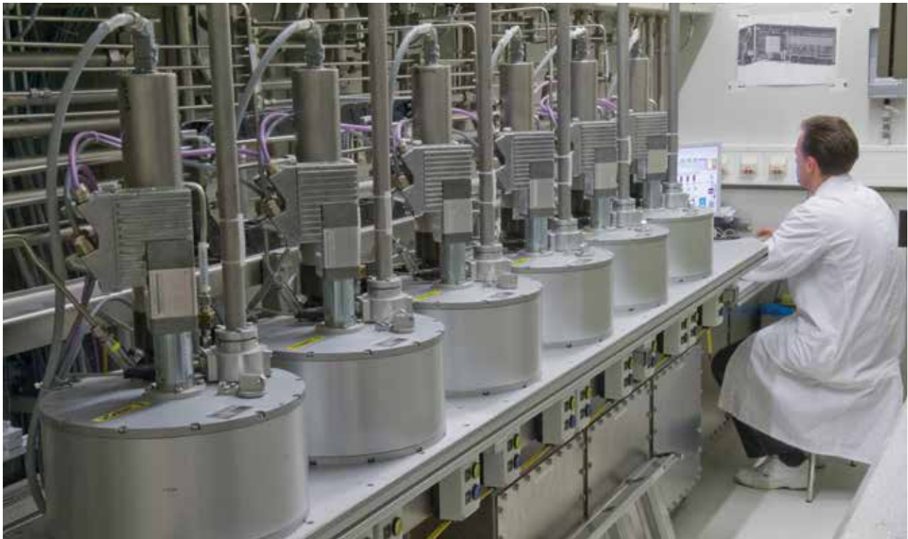
Figure 2: The standard rabbit irradiation system has six independent irradiation channels and is operated by carbon-dioxide.
