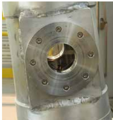
Figure 2: Cryostat with sapphire window (in detail on the left).
