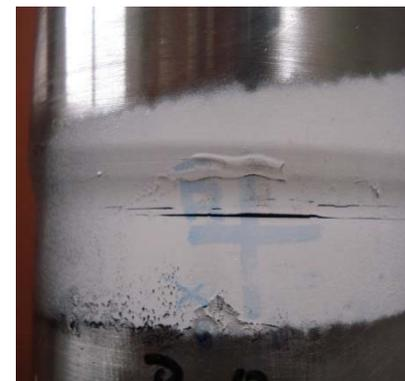
Mini cracks, fatal crack ➔ Fracture mechanics
