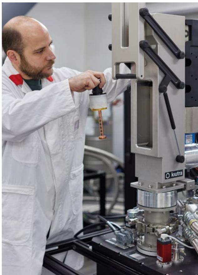
Figure 8: The new ADR cryostat during commissioning activities, with its sample load lock for fast and efficient automated sample mounting.
