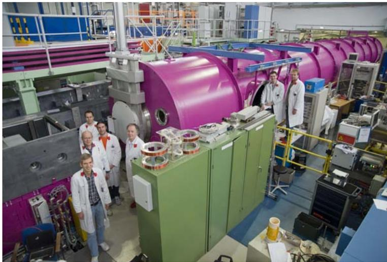
Figure 6.4: Fig. 1: The magenta coloured detector tank of SANS-1 in preparation for the vacuum test.
