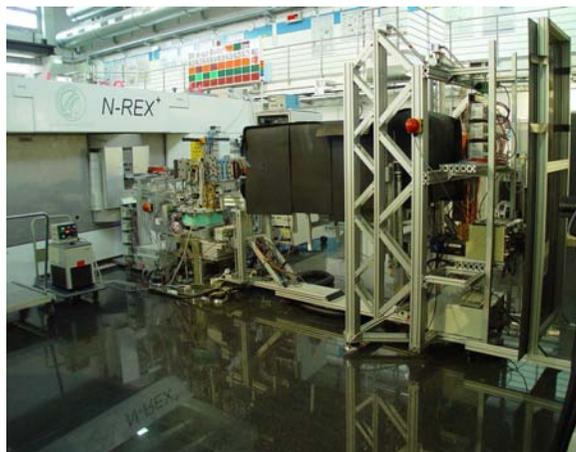
Figure 6.11: The reflectometer N-REX<sup>+</sup> in polarized neutron reflectometry configuration
