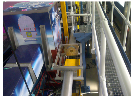
Fig. 1c: Place for 2 T vertical electro magnet at the KWS-3 sample position.
