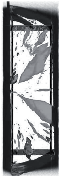
Fig. 1: Distribution of PEG in wood derived from neutron attenuation.
