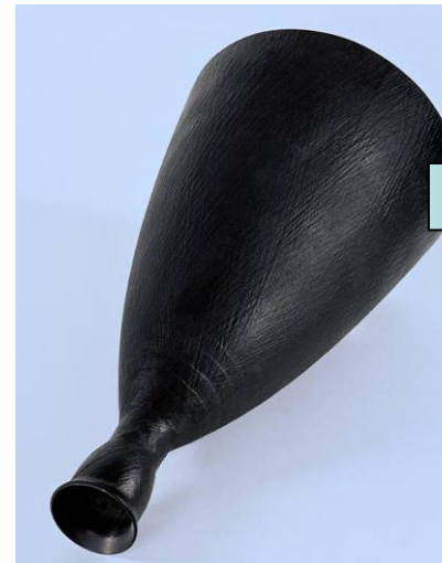
EAM – European Apogee-Motor (Brennkammer & Düse)
