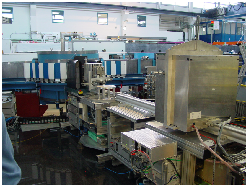
Figure 17.6: MIRA with the second beam port for neutrons with a wavelength of 3-6 Å .
