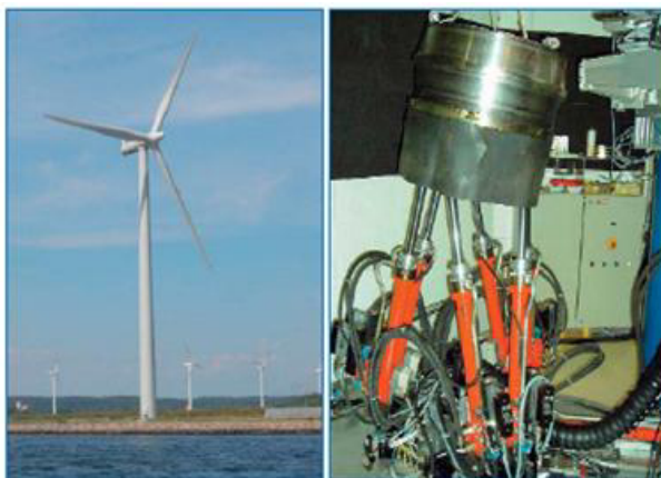
Figure 17.2: SALSA hosting a 600 mm diameter bearing of a wind turbine for tri axial stress determination in bulk and very near surface.
