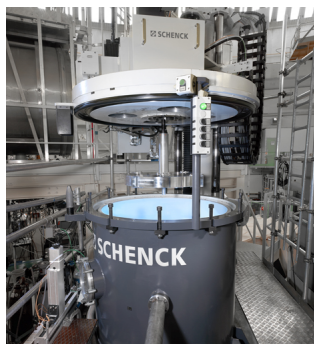
Figure 3.2: Fig. 1: The phase-space transformer installed at the UCN source PF2 (ILL, Grenoble).
