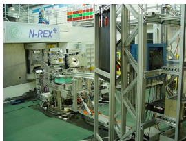
Figure 3.4: N-REX+ - The neutron / X-ray contrast reflectometer with spin-echo option
