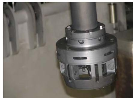
Figure 8.3: new design of the coupler for the sample container.
