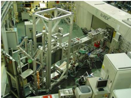
Figure 2.13: N-REX<sup>+</sup> in neutron resonance spin-echo operation mode, with the neutron monochromator hutch on the right and the detector tower on the left.
