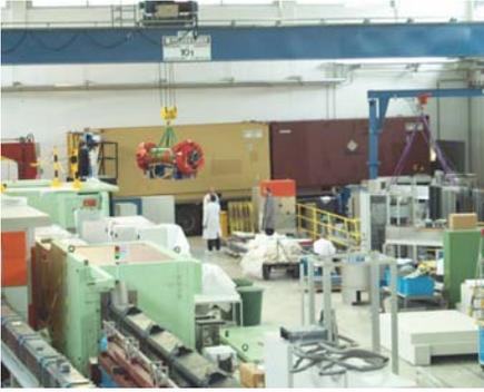
Figure 4.2: One of the two main precession coils of the J-NSE spectrometer entering the neutron guide hall
