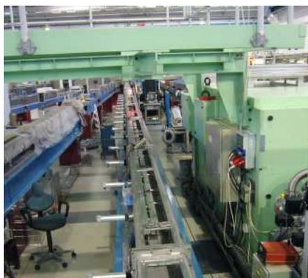
Figure 2.1: View along the KWS-2 collimation housing and mechanical components of the collimation system; to the left the collimation housing of the KWS-1 instrument can be seen.
