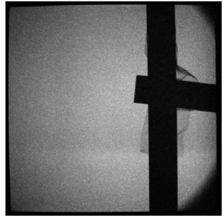
Figure 6.7: The cold source at 3 MW with polyethylen strips in the beam, with the geometric center marked by the upper corner of the horizontal strip.
