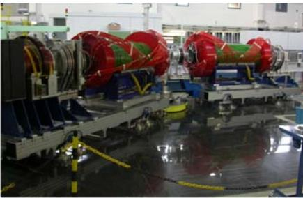
Figure 4.3: The NSE spectrometer during installation in the neutron guide hall.
