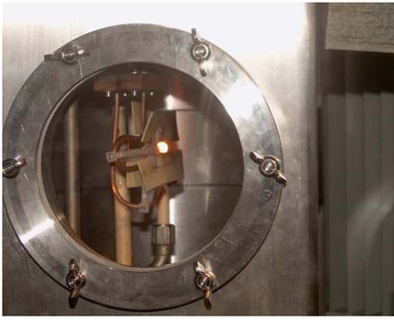
Figure 9.12: Electromagnetically levitated liquid Ni droplet at a temperature of 1810 K. The water cooled copper coil is shielded with a neutron absorbing rubber. The radial collimator of ToF is on the right.
