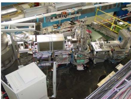
Figure 2.3: MIRA equipped with the MIEZE option, a closed cycle cryostat and a magnet.
