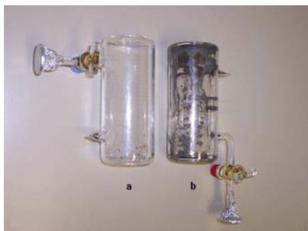
Figure 3.7: a) Spin filter cell *Heidi2*: Small metallic Cs droplets in the lower part of the cell and in the appendix are visible; b) Cell *Heidi1*: The dark spots inside the cell are traces of Cs sub-oxide which is liquid at room temperature.
