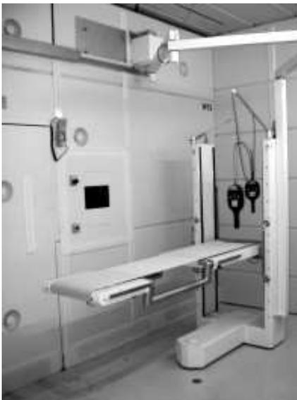
Figure 8.5: Medical irradiation room with treatment couch. The fixed horizontal beam enters from left, 1.45 m above the floor.
