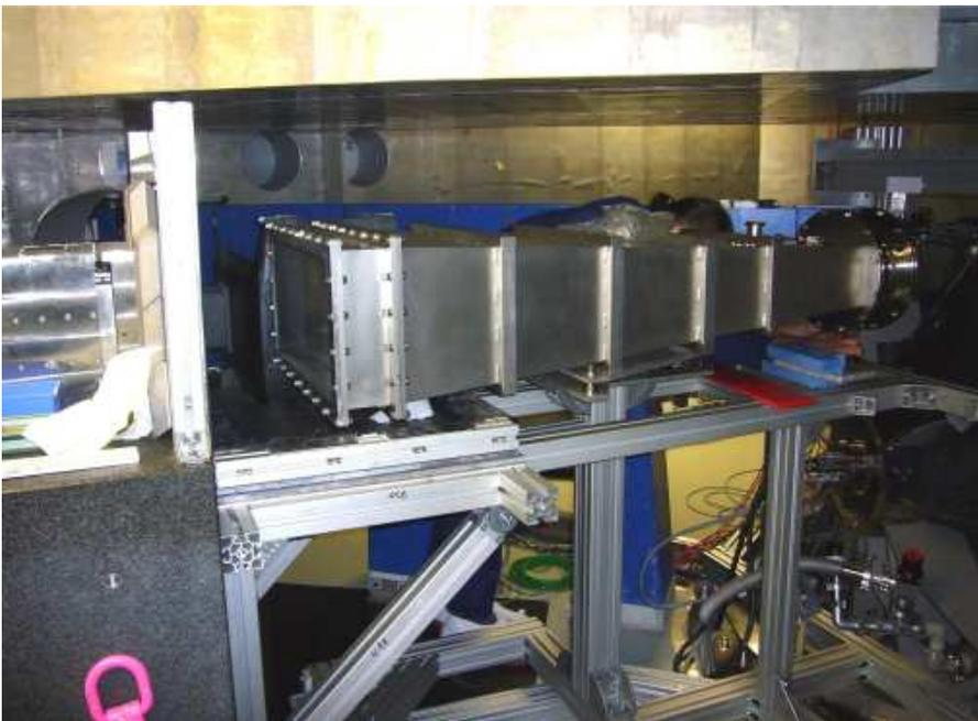
Figure 4.7: Newly installed vacuum flight chamber between the PST chopper (right side) and the Doppler monochromator (left side).
