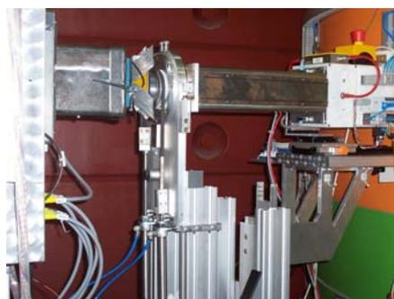
Figure 3.9: Magnetostatic cavity *MB2* fixed on the rotating flange permitting  $180^\circ$  “flipping”
