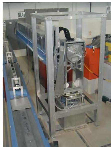
Figure 2.17: First selector installed on site in a Z/tilt stage. (Shielding not shown in this picture).
