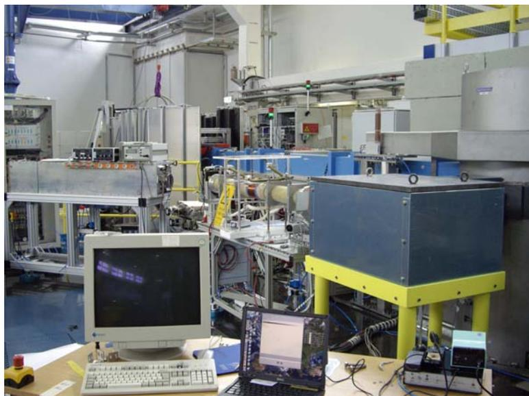
Figure 2.20: TREFF@NOSPEC: From the cylindrical shielding of the first monochromator (right) the neutrons are brought to the shielding box of the second monochromator. Then follows the collimation (with the resonance spin flipper coil around the vacuum tube), the sample table and the detector arm (middle left).
