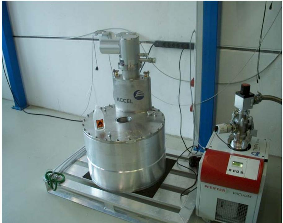
Figure 1.9: 7.5 cryogenfree magnet
