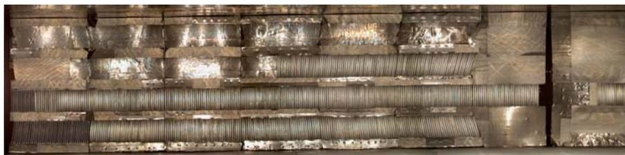
Figure 4.11: Panorama of the detector bank of the TOFTOF spectrometer. The detectors are oriented tangentially to the intersection line of the Debye-Scherrer cones and a virtual sphere with a radius of 4 m around the sample position. Beside the detectors only cadmium sheets are visible shielding the detectors against neutrons not coming from the direction of the sample position.
