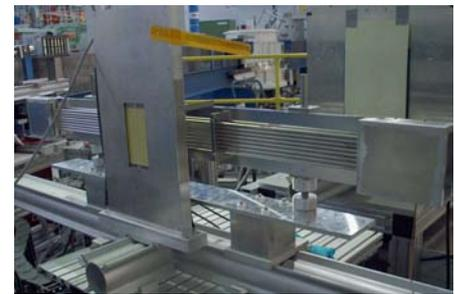
Figure 1.4: A SANS1 prototype detector built of individual  $^3\text{He}$  PSD's mounted at MIRA
