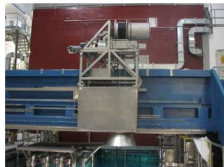
Figure 8.2: lifting unit of the doping facility mounted on the handling bridge.
