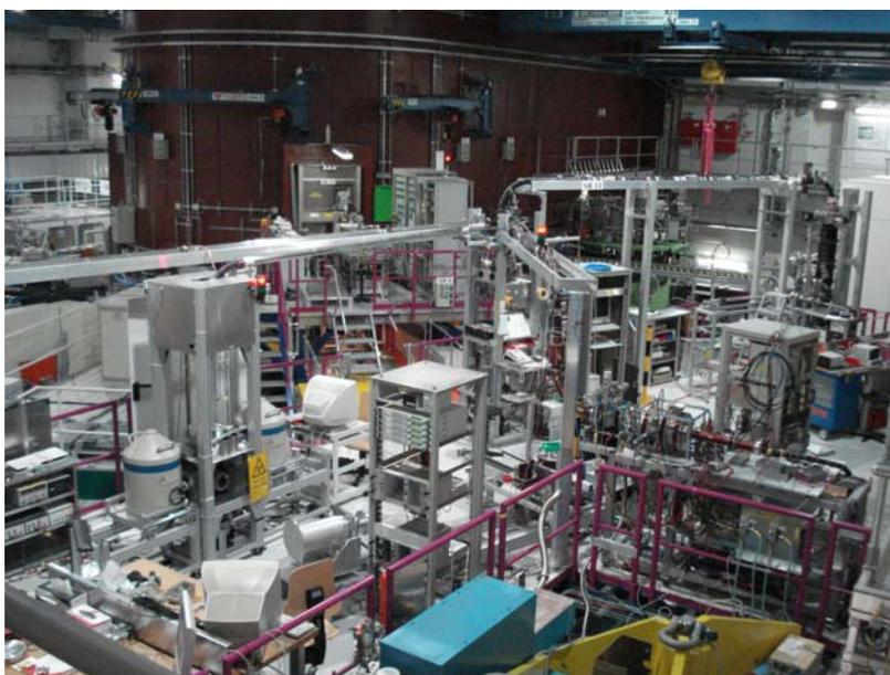
Figure 7.1: The positron beam facility NEPOMUC and positron spectrometers in the experimental hall of FRM II: CDB spectrometer (TUM), PAES-facility (TUM, not shown), apparatus for  $\text{Ps}^-$ -production (MPI nuclear physics, Heidelberg), and components of the pulsed-beam facility PLEPS (UniBw, Munich).
