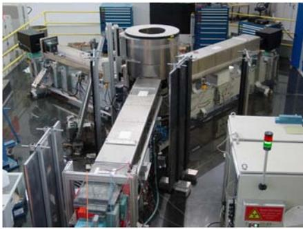
Figure 4.5: The instrument RESEDA with its two secondary spectrometer arms. The mu-metal shielding of the left arm is removed and gives free view on the NSE and NRSE coils.
