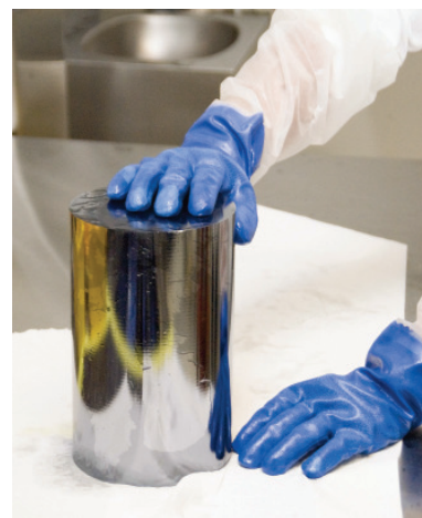
A silicon crystal after the doping.
