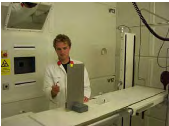
Harald Breikreutz at the medical irradiation facility MEDAPP at FRM II with a sample to analyze the neutron spectrum of the beam.
