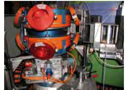
Fig. 2: Picture of the vector guide field coil setup mounted on PANDA.
