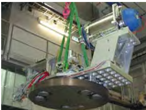
In the experimental hall of FRM II: Transporting the new POLI-HEiDi goniometer basis with mounted detector-analyzer.
