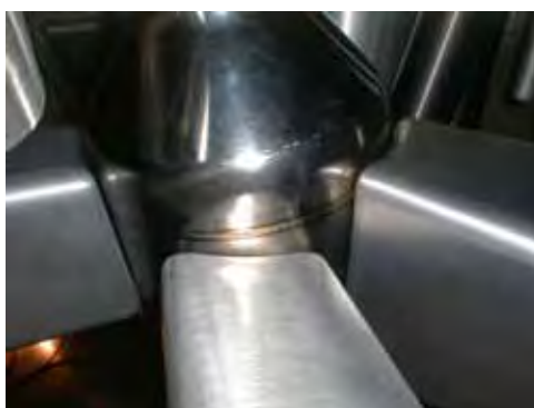
The noses of three beam tubes point to the vessel of the cold source. It contains liquid deuterium.
