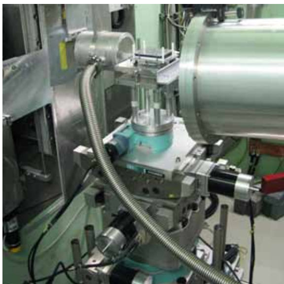
Fig. 1: Sample position of the REFANS instrument with sample cell in place. Evacuated detector tube and primary beam tube are positioned close to the sample to suppress air scattering.
