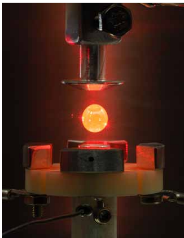
Fig. 1: Electrostatically levitated freely suspended liquid \text{Ti}_{39.5}\text{Zr}_{39.5}\text{Ni}_{21} droplet with a mass of 0.6 g at a temperature of 1150 K.
