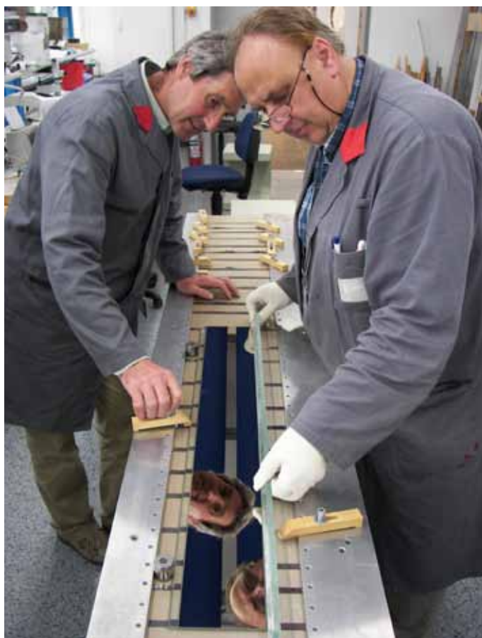
Fig. 3: Josef Weber (left) and Eberhard Kahle (right) prepare a newly sputtered glass for a neutron guide on the bonding table.
