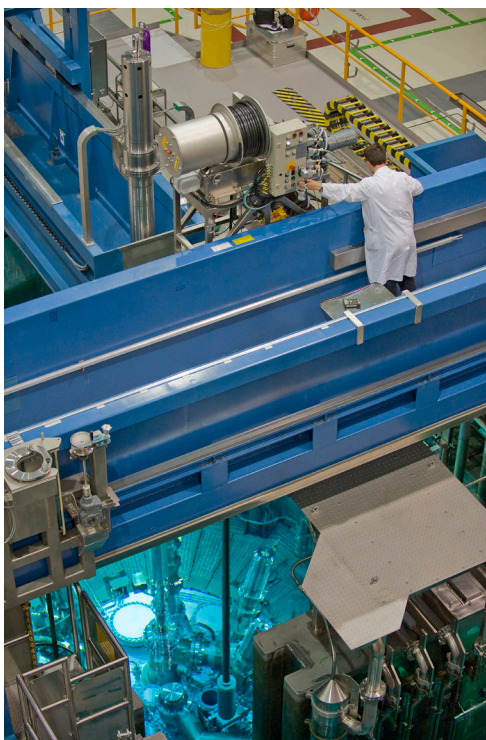
Figure 1: The silicon doping facility at the FRM II, while transporting a silicon crystal under water.
