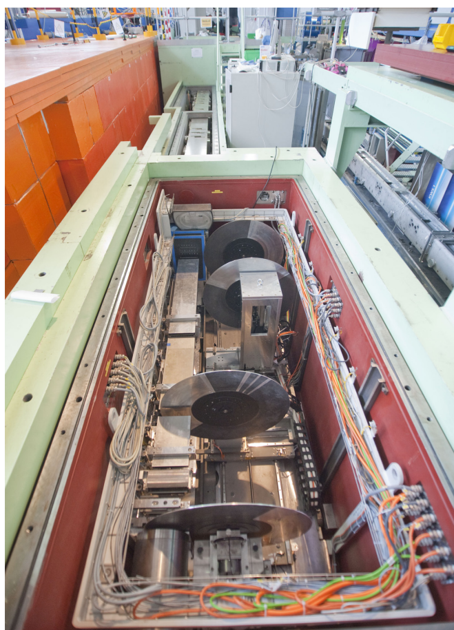
Figure 1: The chopper chamber of REFSANS during the test phase. The master disks are inserted in the guide while the slave disks are on a parking position outside of the beam path (view from reactor to sample).
