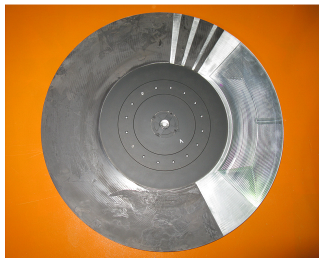
Figure 2: One of the master disks. The black absorbing material defines several windows to enable different chopping schemes.
