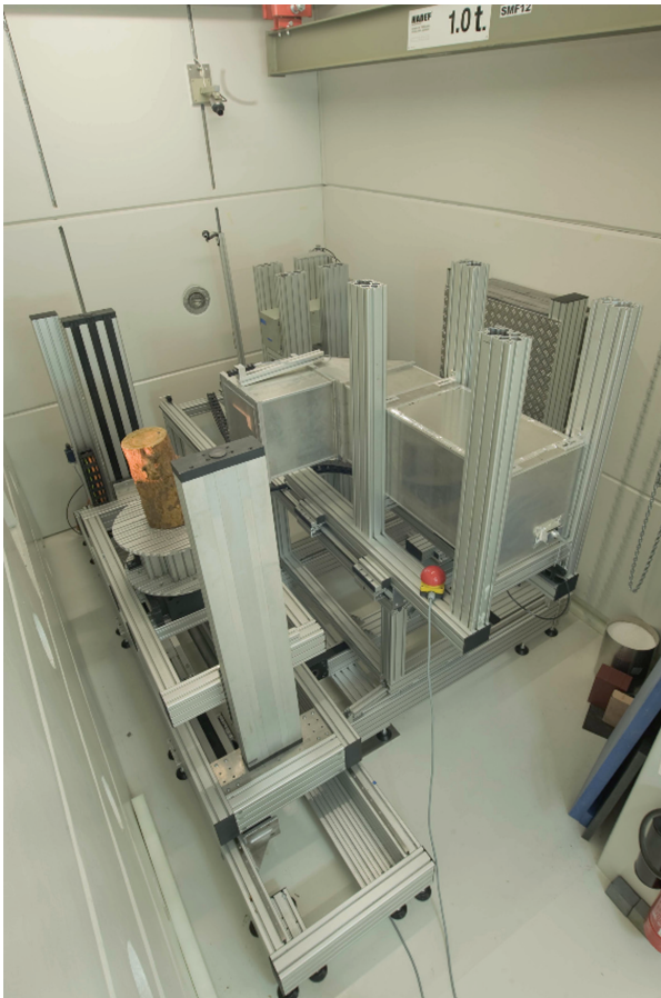
Fig. 1: Measuring room of NECTAR with a wooden sample on the turntable.
