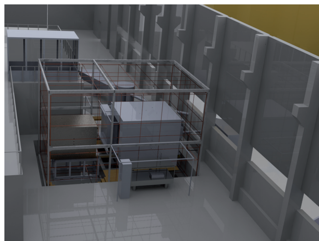
Fig. 3: Artist's view of the EDM installation in the neutron guide hall east. The experiment itself is placed inside a magnetically shielded room (grey box with sliding door). The inner magnetic field is mounted on rails and can slide into the shielded room. A 3D arrangement of field coils surrounds the assembly.
