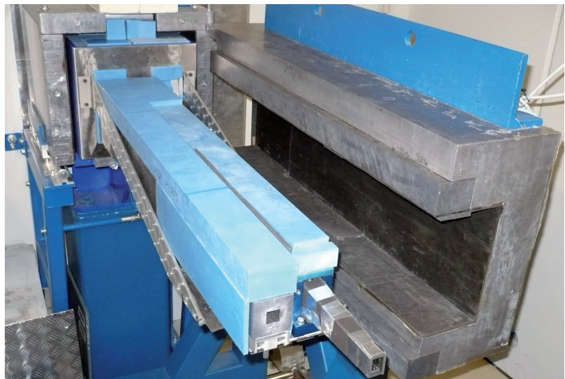
Fig. 2: Beam collimator and elliptical neutron guide, shielded.
