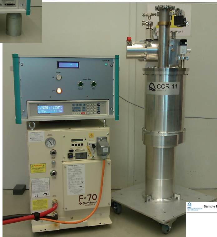
Fig. 2: Combination of control box (top), compressor (bottom) and CCR.
