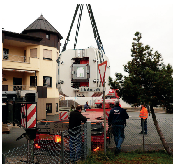
Fig. 1-2: SAPHiR starting its way to Garching in Mainleus, Oberfranken. Above: The positioning table. Below: Loading of the 50 ton multianvil press.
