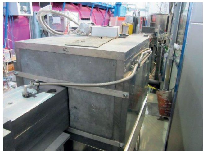
Fig. 2: View from the exit of the neutron guide NL5-S towards the instrument. The new velocity selector housing appears in the grey box in the middle.
