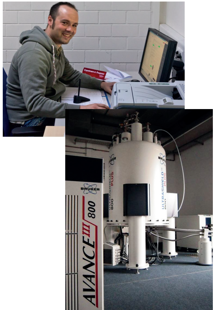
Fig. 4: Janosch Hennig navigating an 800 MHz (18.8 T) NMR spectrometer (bottom). The combination of NMR and SANS data (which can be recorded at FRM II) boosts structural biology research to new heights.
