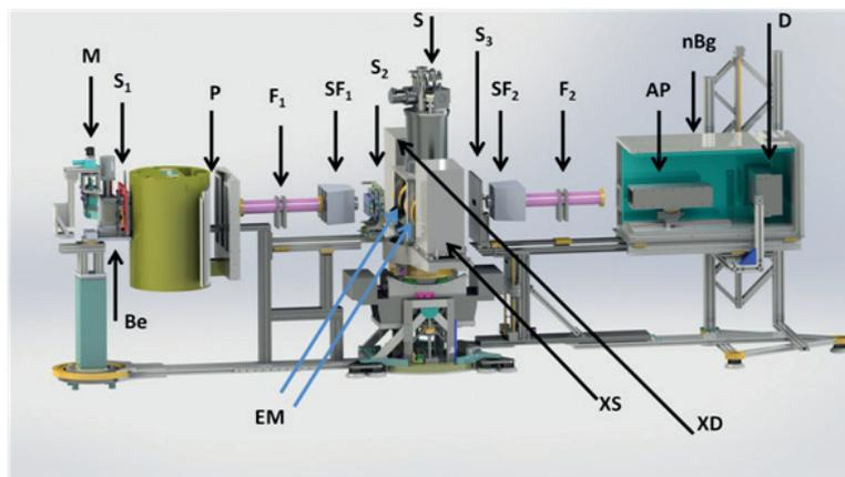
Fig. 1: Scheme of NREX. **M** = monochromator, **Be** = beryllium filter, **S1-S4** = slits, **P** = polarizer, **SF1, SF2** = spin flippers, **S** = sample goniometer, **EM** = electromagnet, **nBg** = background shielding, **AP** = analyzer, **D** = neutron detector. **X** = ray part (works without magnet): **XS** = X-ray source, **XD** = X-ray detector.
