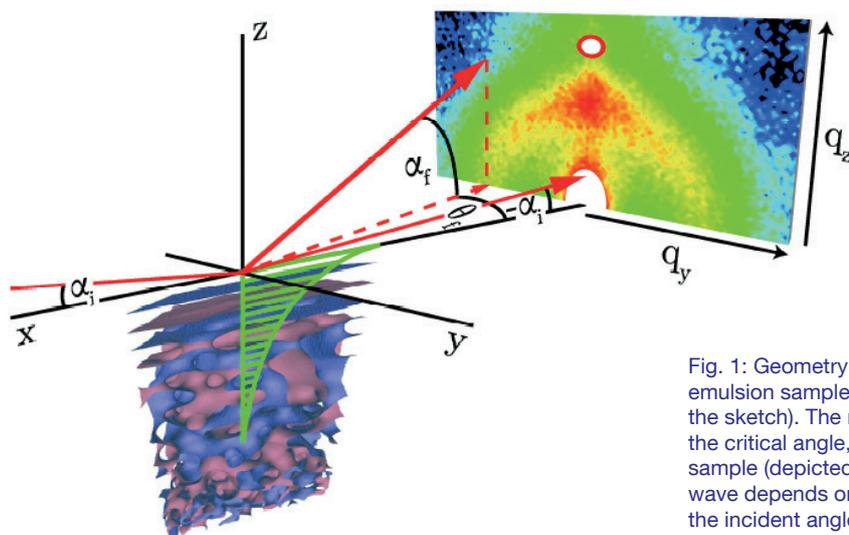
Fig. 1: Geometry of the GINSES experiment for a bicontinuous microemulsion sample close to the rigid Si interface (on top, not shown in the sketch). The neutron beam hits the sample with an angle below the critical angle, and an evanescent neutron wave is penetrating the sample (depicted in green). The scattering depth of the evanescent wave depends on the contrast between sample and Si-block and on the incident angle.
