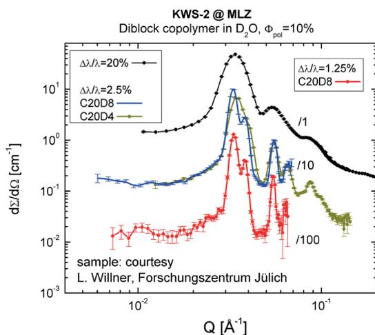
Fig. 2: Measurements with variable resolution carried out on structures formed by a n-alkyl-PEO system in D<sub>2</sub>O, at high polymer volume fraction.
