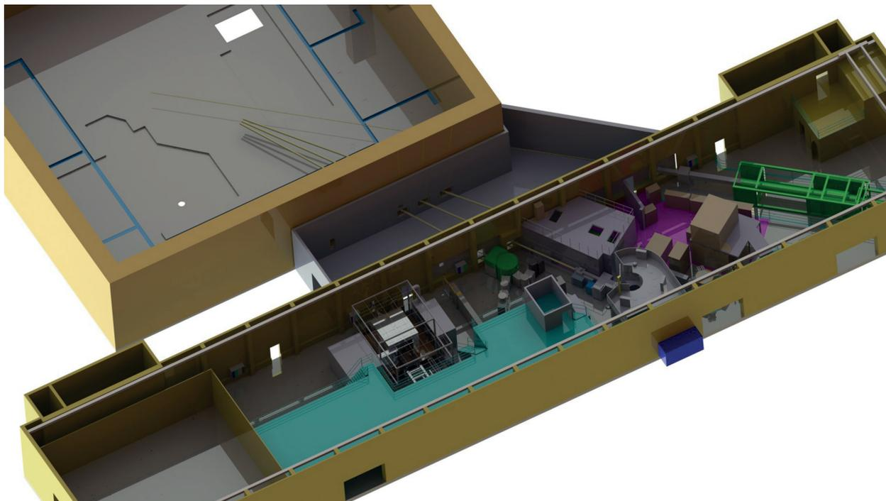
building. This new building hosts a major part of the neutron guide system including beam conditioning devices like choppers. The body shell of the new building will be completed in autumn 2013.
