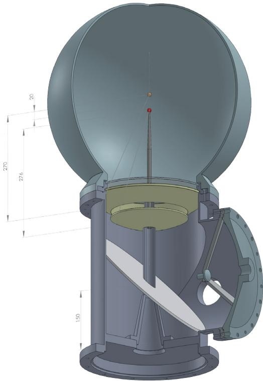
Fig. 2: Rotatable recrystallisation furnace with lens system for homogeneous sample heating by a (pulsed) laser. The furnace can either be evacuated or used as 'flow-through' furnace for different noble gas atmospheres. Construction and image by Herbert Weiss, FRM II, Garching bei München.
