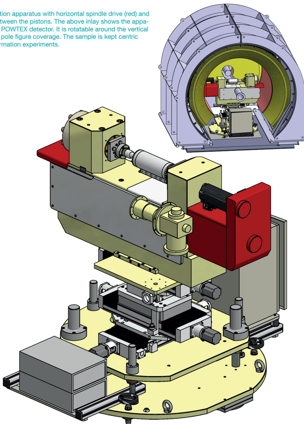
op sample environments for in-situ experiments at the new POWTEX (**POW**der and **TEX**ture) diffractometer at FRM II, because neutron diffraction is the only method which allows bulk texture analysis of several  $\text{cm}^3$  sample volumes.
