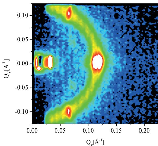
GISANS soft-matter measurement with 10  $\text{\AA}$  in 1200 s of  $\text{C}_{10}\text{E}_4$  +  $\text{Pep}_{15}\text{Peo}_5$  on a silicon surface in the hexagonal phase.
