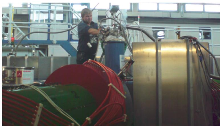
Fig. 2: Harald Schneider working hard to provide 25 mK at the J-NSE. During this experiment, the J-NSE has been the coolest place in the neutron guide hall. In this example nuclear spin waves of a  $\text{Nd}_2\text{CuO}_4$  crystal were investigated.
