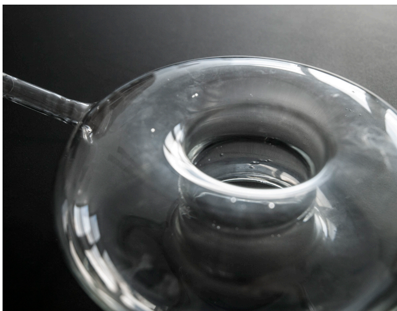
Fig. 6: Doughnut shaped ^3\text{He} polarisation cell ( \varnothing 20 \text{ cm} \times 8 \text{ cm} ).
